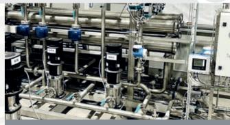
Our special design permits to reach very high recovery ratio (more than 90%) with optimal quality for direct reutilization.
